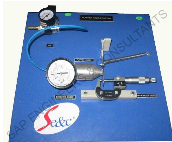
FLAPPER NOZZLE ASSEMBLY TRAINER (SAP – 21)
